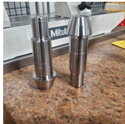
The finished pinion blank.
