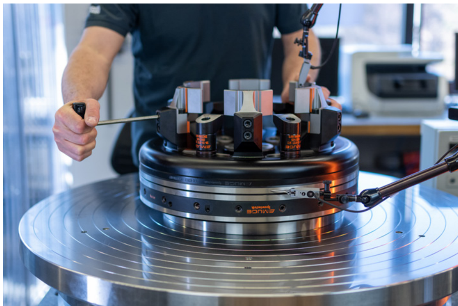
Designed with indicating in the base and jaws on a diaphragm for perfect runout correlation between the two.
