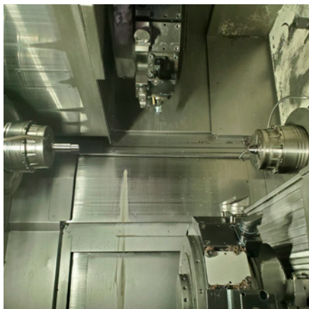
Main/Sub Spindle TOPlus mini chucks showing (left side pinion shaft, right side pinion head).
