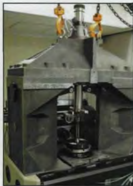
Russell, Holbrook & Henderson's ultra precise gear measuring machine certifies the accuracy of gears within 0.1-0.3 μm.
