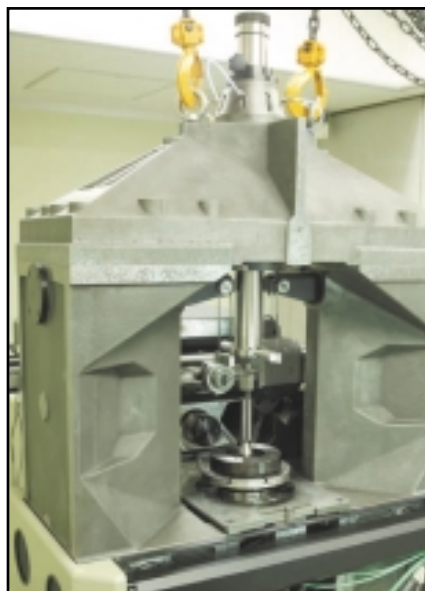
Russell, Holbrook & Henderson's ultra precise gear measuring machine certifies the accuracy of gears within 0.1–0.3 \mu m.
