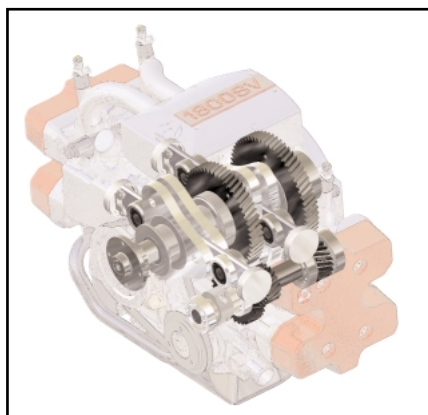
An Engine Block with Gears —Inside the engine block are five helical gears that transfer part of the engine's power to its output shaft.
