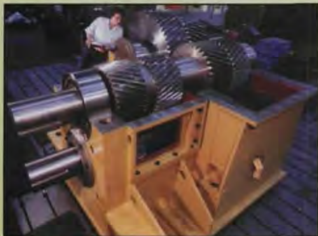
A cold mill combination speed increaser/pinion stand.
