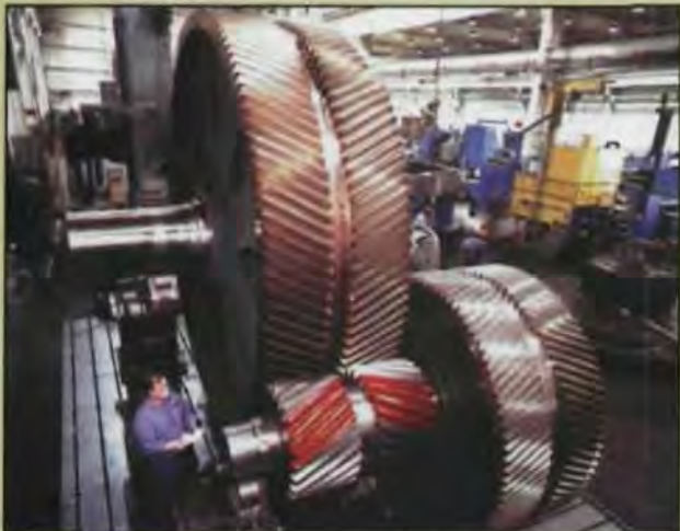
A double helical gear set for the main drive of a hot strip mill, undergoing final mesh test at Horsburgh & Scott.
