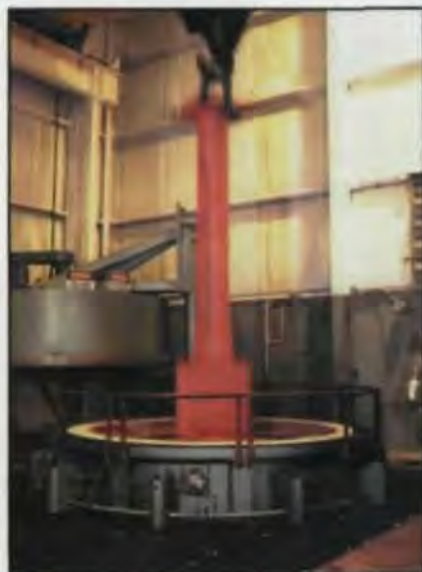
Horsburgh & Scott's carburizing furnaces can handle parts up to 75" in diameter and 180" long.
