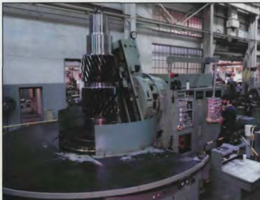
Maag hard cutting is a specialty at Horsburgh & Scott. Using a CBN tool, the company cuts hardened gears "as accurate and smooth as a ground gear," says president Dave Kraninger.
