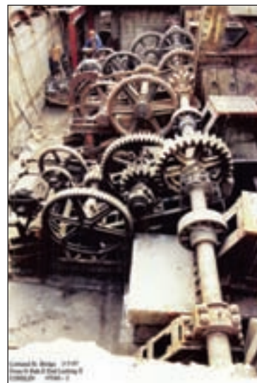
A look at the gear set that powers the Cortland Street Bridge. (Photo courtesy City of Chicago.)
