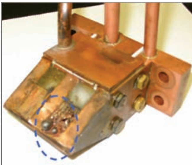
Figure 6—Typical coil failure of a gap-by-gap inductor.
