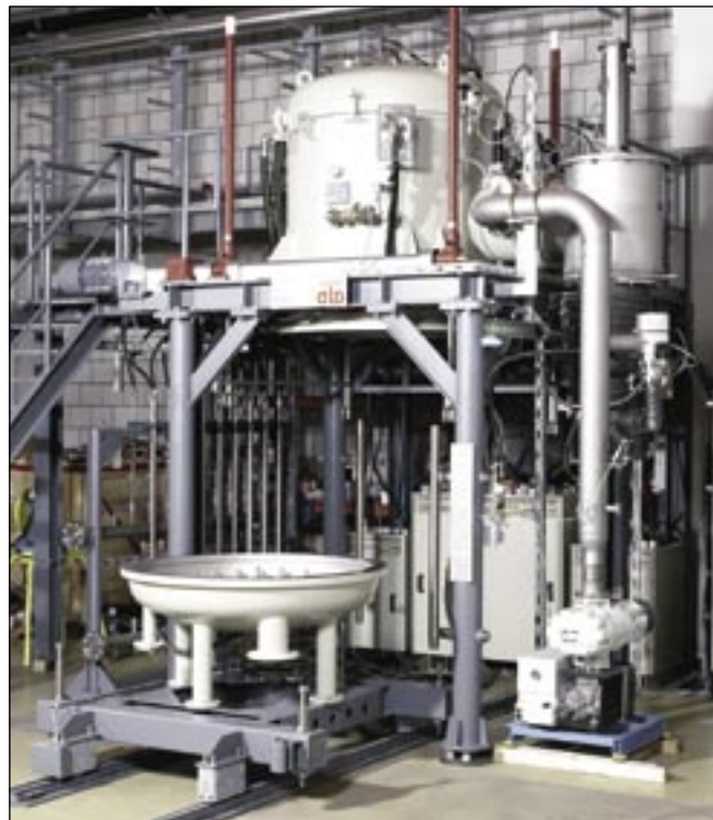
Figure 3—Bottom loader for LPC of large parts with integral gas quench.
