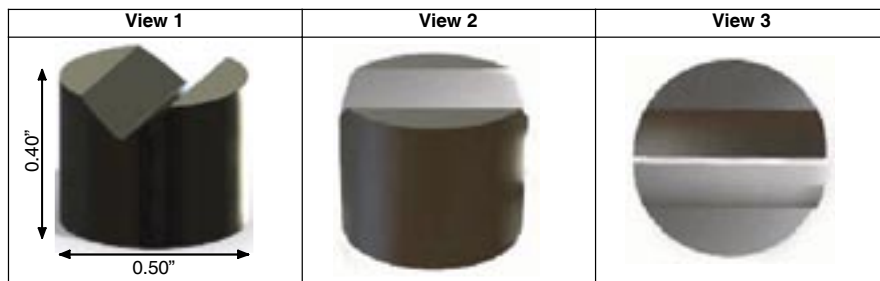
Figure 2—Drawings of Falex V-Block showing three different views.
