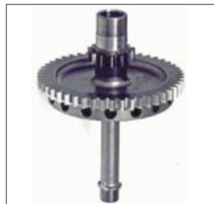
Figure 9—As-received used/scrap carburized AISI 9310 gasifier train gearshaft.
