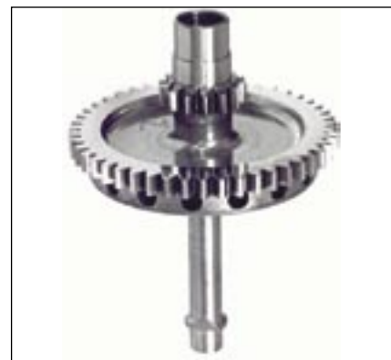
Figure 10—Superfinished used/scrap carburized AISI 9310 gasifier train gearshaft.
