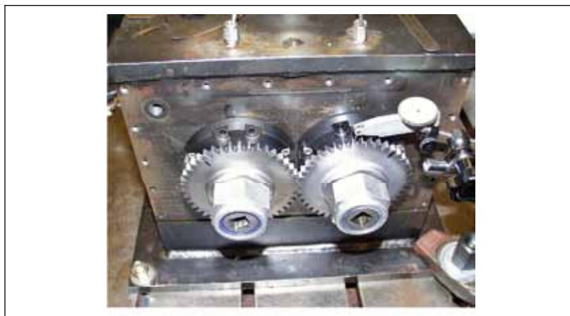
Figure 2—Set-up for backlash measurement using dial indicator.
