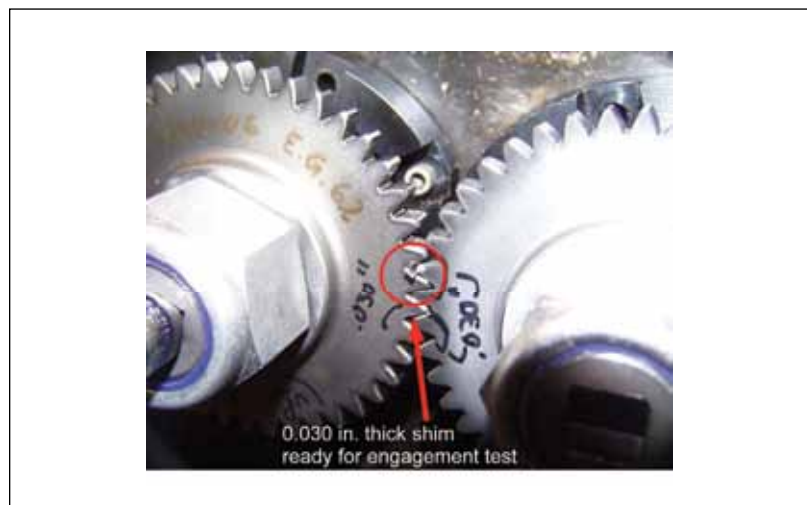
Figure 3—Example of shim and placement used for engagement testing.
