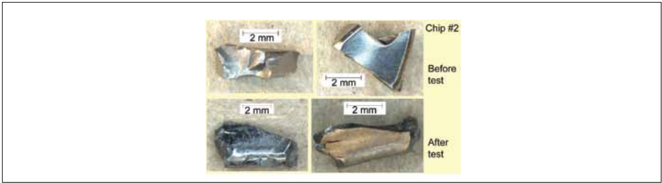
Figure 10—Chip #2, mass of chip 0.100 grams.
