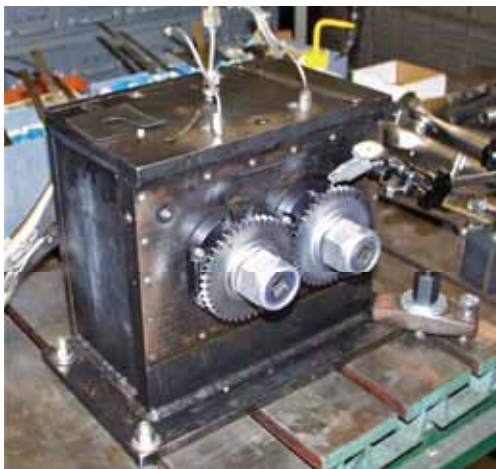
Figure 1—Bench set-up for gear chip engagement testing using the NASA Glenn fatigue rig.
