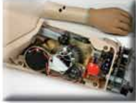
Articulating gear for the electric terminal device on the Utah Arm... patient can tie his shoes
