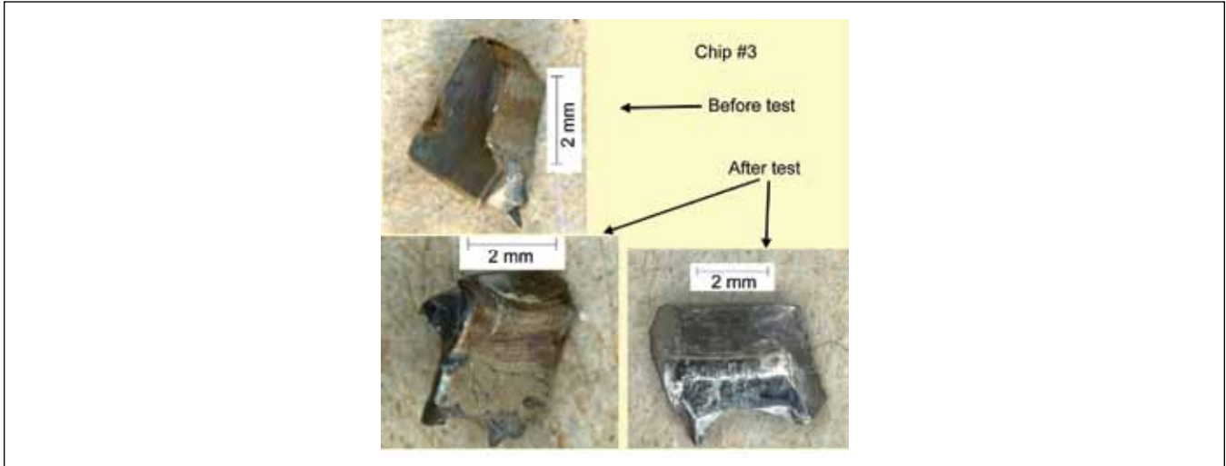
Figure 11—Chip #3, mass of chip 0.106 grams.
