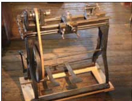
This metal working lathe with two foot pedals was donated by the Carroll-Jamieson Machine Tool Company in Batavia, OH.
