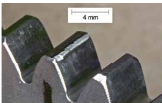
Figure 6—Example of damaged tooth tip after engagement of 1.96 mm (0.077 in.) diameter drill bit shank.
