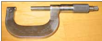
This micrometer was made by Brown & Sharpe Mfg Co., Providence, RI, and was a gift from Charles W. Dodge (courtesy of the American Precision Museum).
