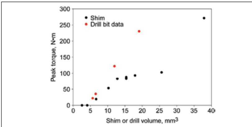
**Figure 4—Relationship of volume of engaged objects to the peak torque required to rotate the gears for the NASA GRC spur gear rig using 12-pitch case-carburized steel gears.**
