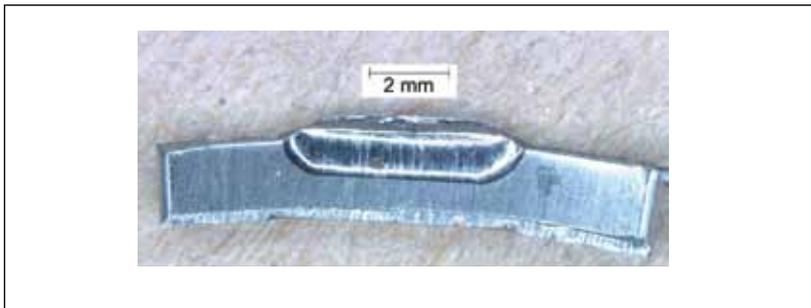
**Figure 5—Example of deformed shim stock after engagement of meshing gear teeth.**
