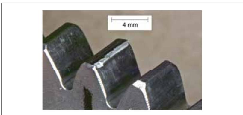
**Figure 6—Example of damaged tooth tip after engagement of 1.96 mm (0.077 in.) diameter drill bit shank.**
