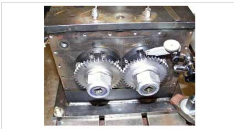
Figure 2—Set-up for backlash measurement using dial indicator.
