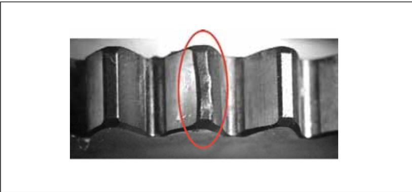
**Figure 8—Severely deformed gear tooth as a result of engagement with largest chip tested, chip #7 having a mass of 0.342 grams. The gears can no longer be rotated to engage and pass through this tooth after using hand torque.**
