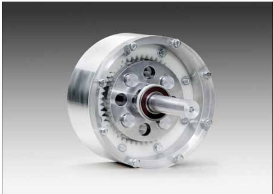
The plastic transmission design gives Winzeler Gear a prototype for which they can build a business case.
