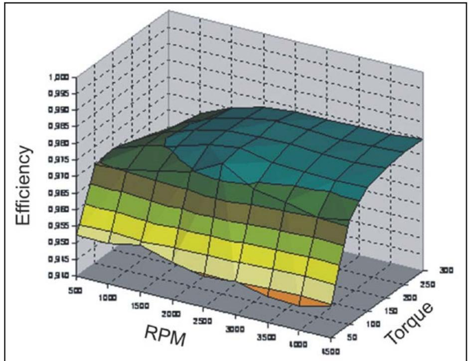
Figure 1 Efficiency characteristics versus speed and torque.
