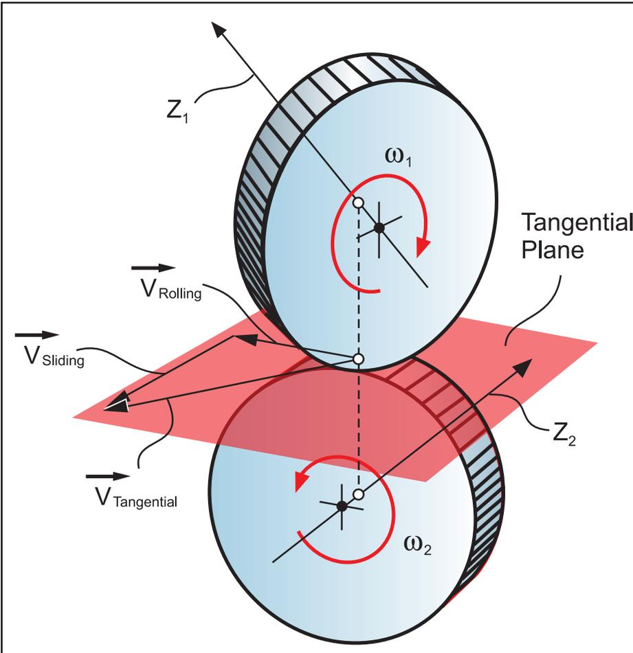
Figure 5 Definition of sliding and rolling velocity.
