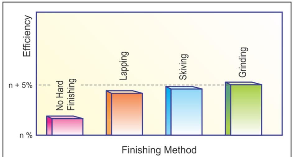
**Figure 8** Quantitative comparison of hard-finishing influence with efficiency.
