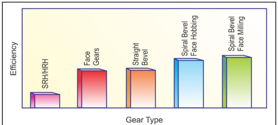
**Figure 9** Quantitative comparison of different gear type efficiency.
