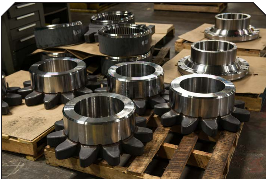
Big gears, fast turns —Snyder Industries manufactures gears ranging in size from 50-5000 lbs. To reduce lead times the company replaced nearly all of its machining equipment with advanced multi-axis machining centers and CNC lathes with live tooling. The company is actively working to continuously reduce costs and increase productivity by taking full advantage of all the capabilities offered by its CAM software.
