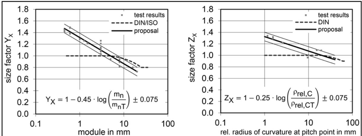
Figure 9 Proposed size factors for tooth bending strength (left) and pitting load capacity (right) for case-hardened steel 16MnCr5 based on test results.
