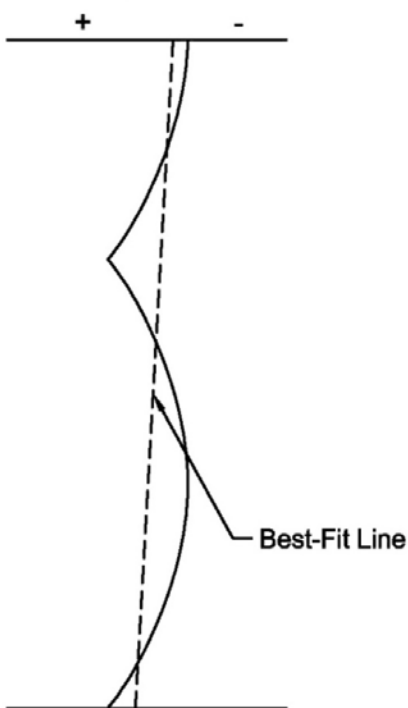
Figure 8 It is extremely important to use a best-fit evaluation for slope deviation, as illustrated above. The use of a simple intersection point evaluation may incorrectly induce slope error and slope variation from tooth to tooth, depending on where the inspection trace crosses the evaluation zone lines.
