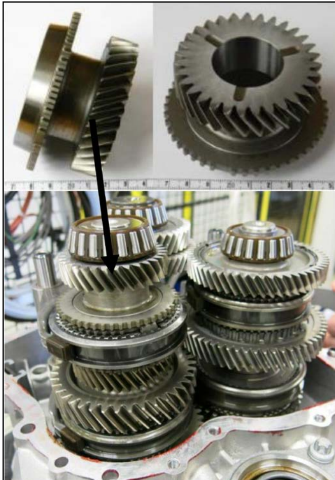
Figure 1 Top: two views of 6th output gear; Bottom: gearbox before case is bolted together; 6:th output gear is clearly seen (see arrow).
