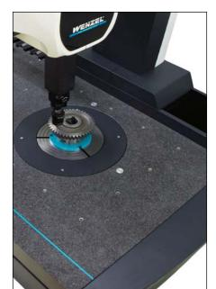
The LH Gear is a gear measuring machine for shops that need something different than a dedicated gear checker. The LH Gear has an attractive entry price to get you started into the gear checking world.
