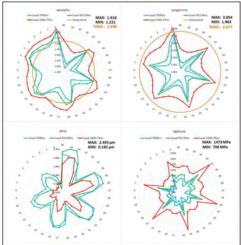
Figure 9 Overview of the main results for 37 profile modification variants at 3 torque levels; profile contact ratio under load \epsilon_\alpha , total contact ratio \epsilon_\gamma , PPTe and maximum Hertzian pressure.
