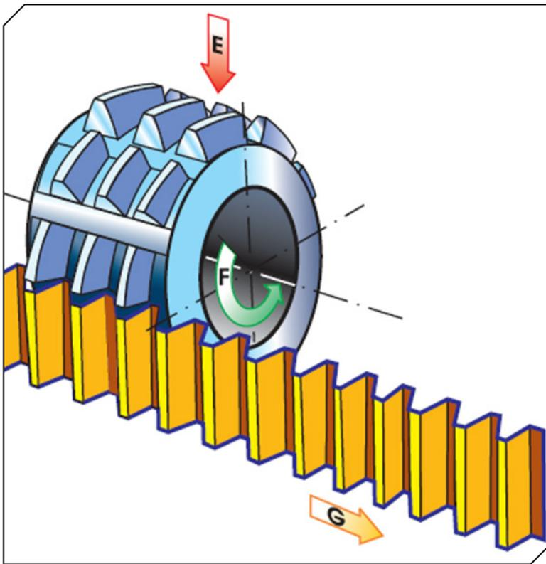
Figure 3 Hob cutter representing the trapezoidal generating profile.
