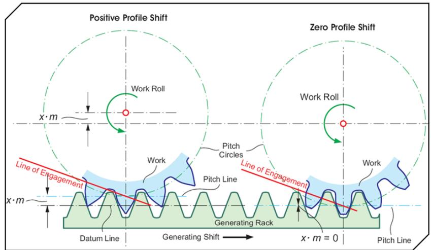
Figure 8 Elimination of undercut with profile shift.
