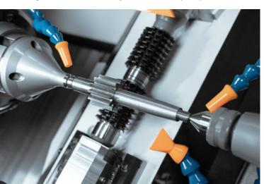
for manufacturing high volumes of automotive pinions and gears. And, if your operation is looking to replace aging manual hobbing machines, EMAG's long-bed version of this multiaxis machine can handle long shafts and heavy gears. Like the standard K 160, it comes with direct-driven performance drives, user-friendly and easy-to-program controls as well as built-in automation.
