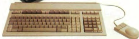
Alpha-numeric keyboard with "Mouse" for one-time entry of part print and tolerance data. "Mouse" permits use of CAD techniques.
