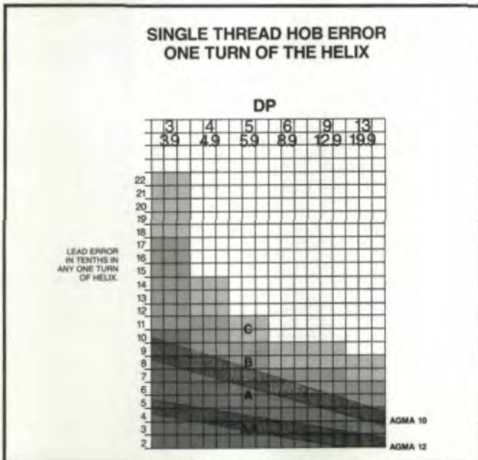
SINGLE THREAD HOB ERROR IN ONE TURN OF HELIX RELATIVE TO HOB CLASS ACCURACY REQUIRED TO PRODUCE INVOLUTE TO AGMA 10 & 12 TOLERANCES FOR 10° TO 20° DIAMETER GEARS.
