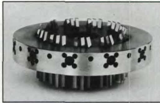
Fig. 10 - Single-part blade head for series manufacture.
