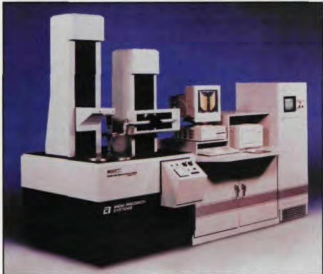
Fig. 1 — M & M Precision's 4-axis, Model 3025 PC gear process control system.
