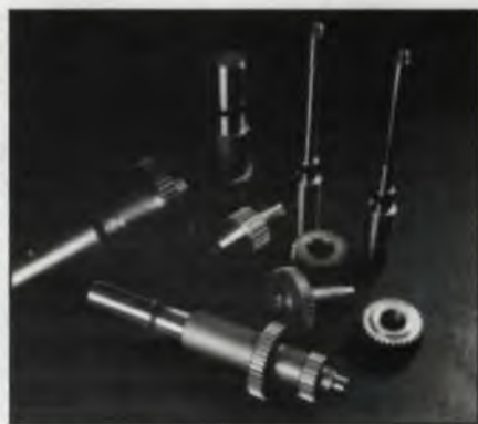
To streamline gear production at Ann Arbor Machine Co., most gears have the same pitch and pressure angles. Gears manufactured are usually straight spur gears and some with internal splines.
