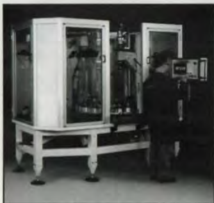
Modular Vertical Honing System (MVH) from Sunnen Products Company.
