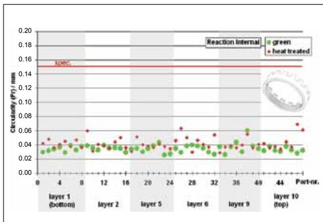
**Figure 12—Circularity of reaction internal gears before and after heat treat (LPC and HPGQ with dynamic quenching); specimen maximum after heat treat—150  $\mu\text{m}$ .**
