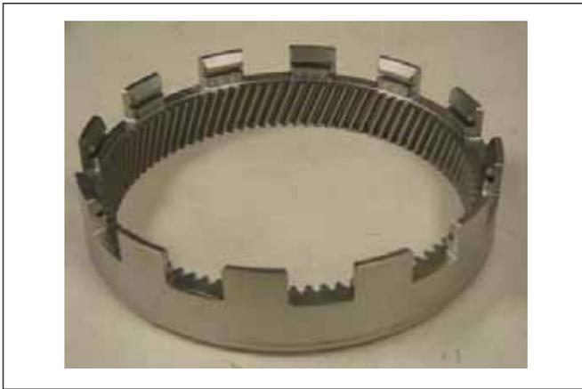
**Figure 8—Input internal gear ( $d = 139$  mm, 89 internal teeth).**
