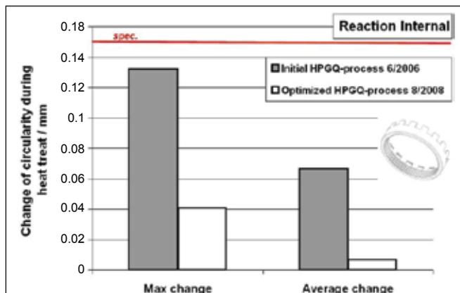
**Figure 15—Maximum and average change of circularity during heat treatment in a load of reaction internal gears; comparison of initial production process from 2006 and the optimized production process used since 2008; specimen maximum after heat treat—150  $\mu\text{m}$ .**
