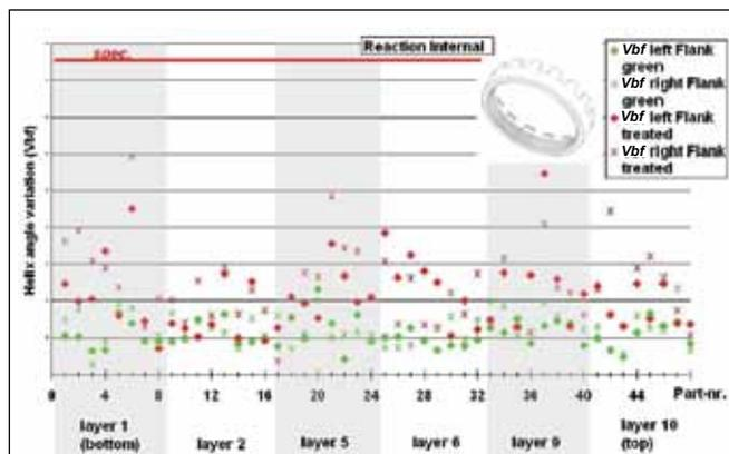
**Figure 14—Helix angle variation of reaction internal gears before and after heat treat (LPC and HPGQ with dynamic quenching).**
