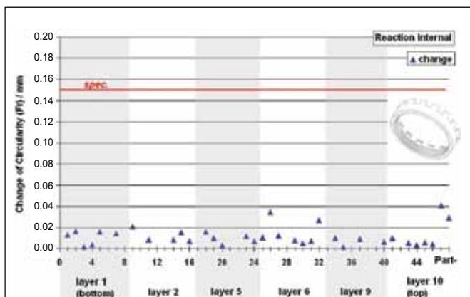
**Figure 13—Change of circularity of reaction internal gears during heat treatment (LPC and HPGQ with dynamic quenching); spec. maximum after heat treat: 150  $\mu\text{m}$ .**
