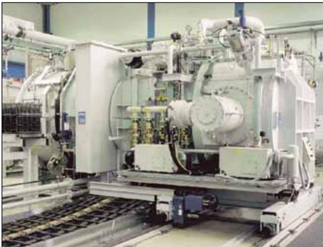
Figure 4—ModulTherm heat treat system with gas quenching chamber.
