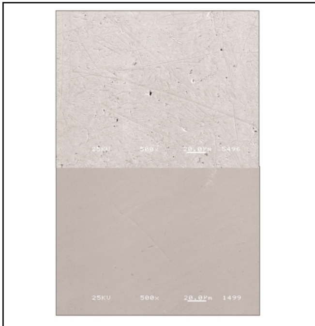
Figure 1—SEM images of test specimens superfinished with ceramic (top) and plastic (bottom) non-abrasive media.
