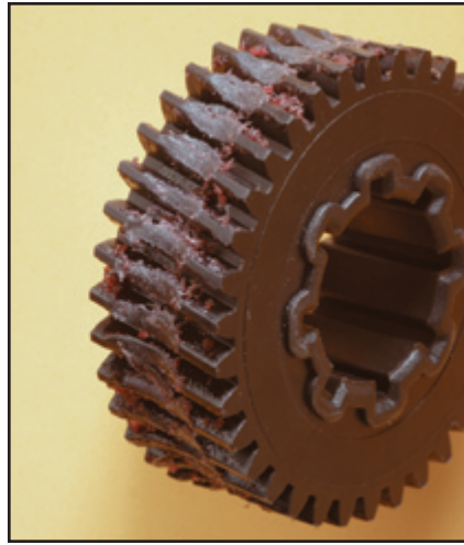
Figure 4—Gear with melted teeth.
