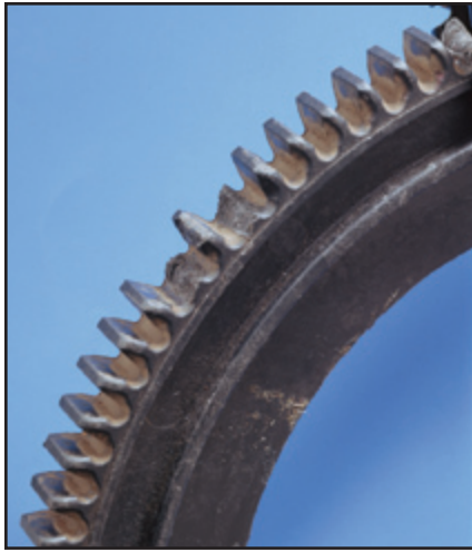
Figure 3—Gear with broken teeth.
