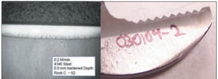
Typical heat treating results with the HighLight laser.
