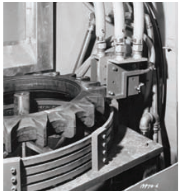
Figure 13—A multi-turn encircling inductor for hardening large gears.
