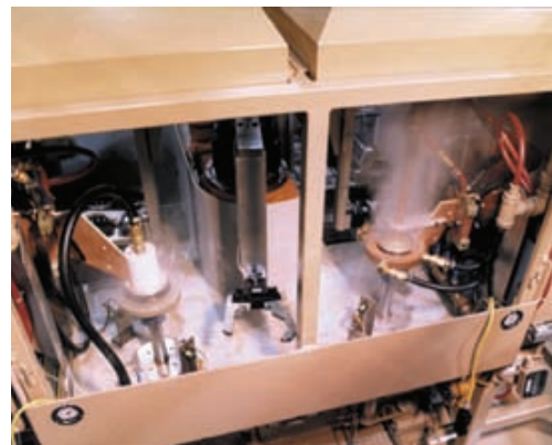
Figure 12—Induction hardening of an automotive transmission component with smaller, helical teeth on the ID and large teeth on the OD.
