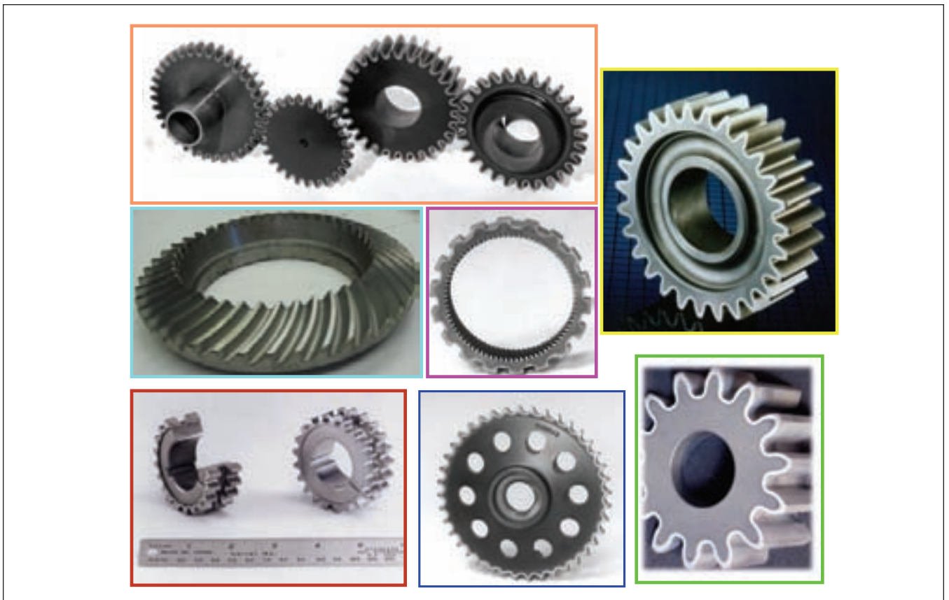
Figure 8—Examples of gears that use spin-hardening techniques.
