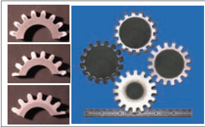
Figure 9—Diversity of hardness patterns obtained with induction spin hardening.
