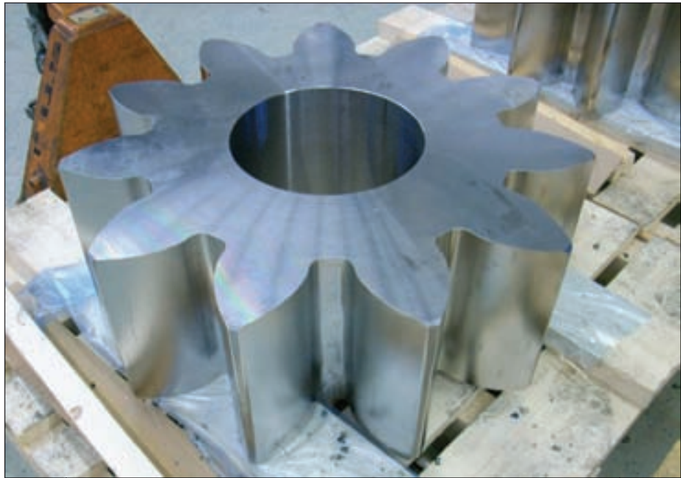
A large spur gear finished using the Depo concept (courtesy of Depo).
