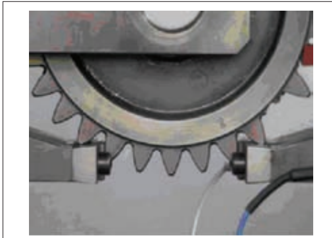
Figure 5—Gear specimen during test.
