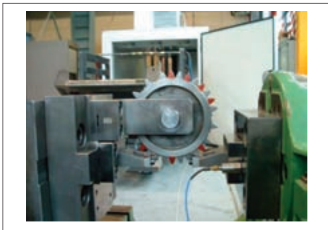
Figure 4—Fixture designed for Agusta-Westland tests.
