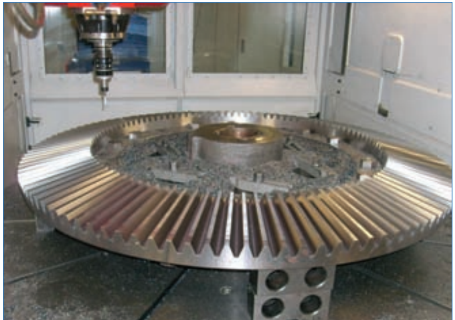
Inspection software from Depo allows for on-the-machine inspection of a large bevel gear (courtesy of Depo).
