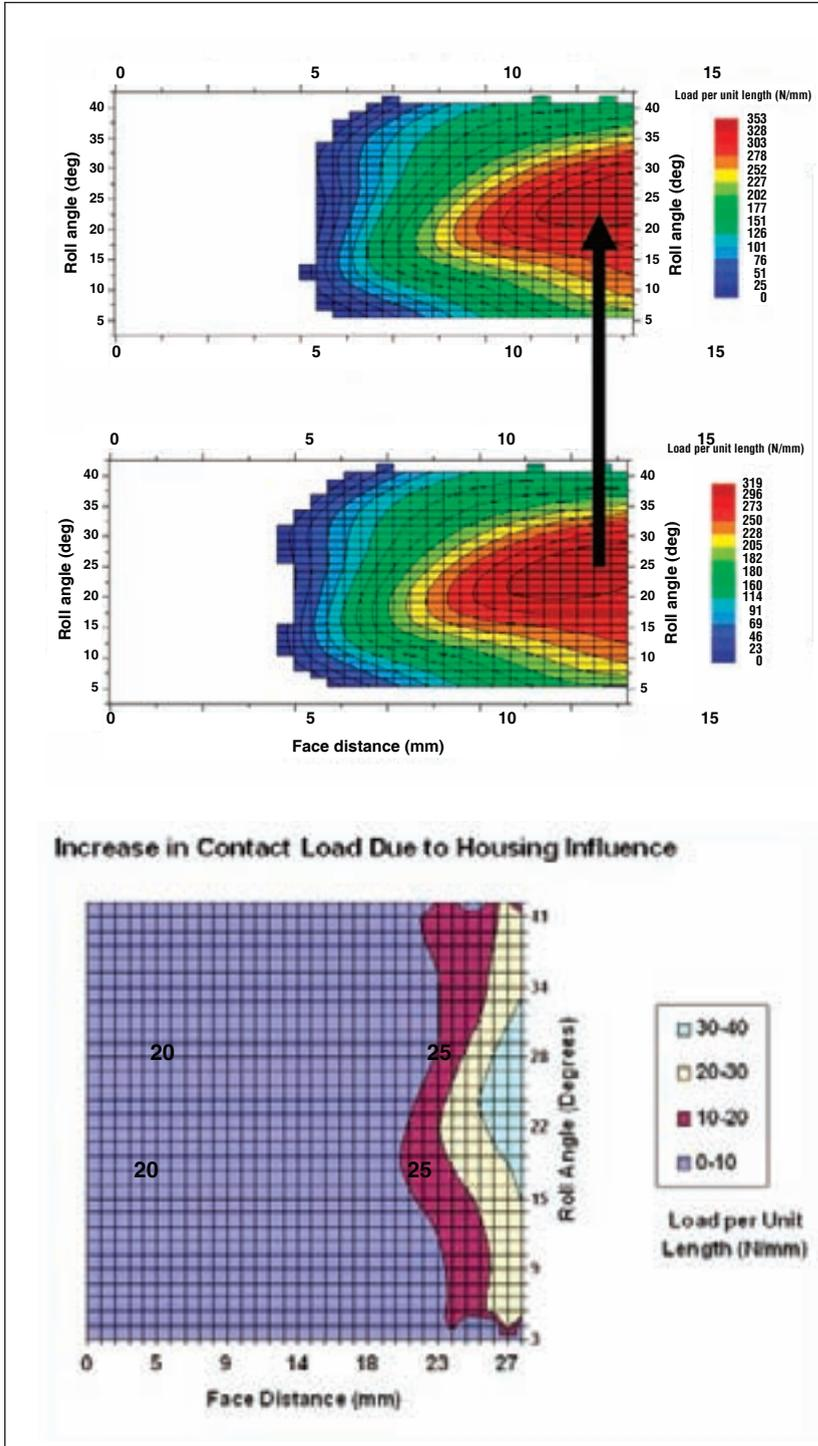
Figure 9—Contact patterns, final drive gear mesh, 400 Nm, with (top) and without (bottom) housing.
