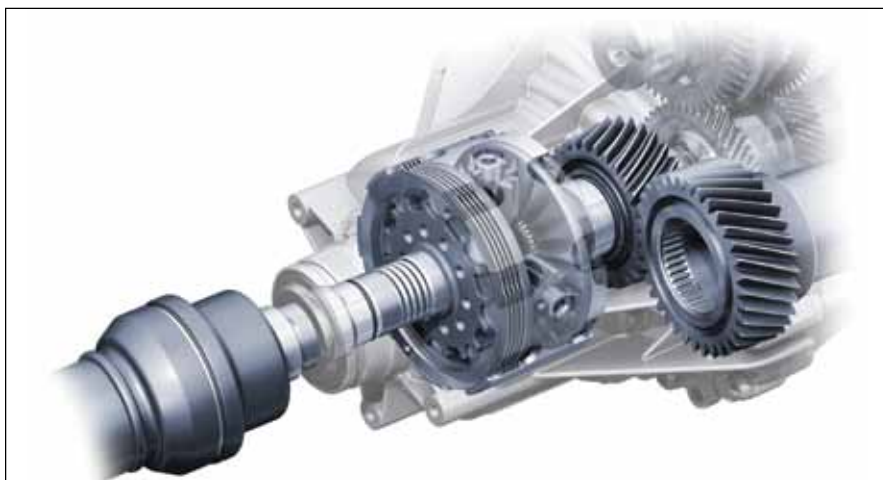
Figure 9—Embedded face gear center differential.
