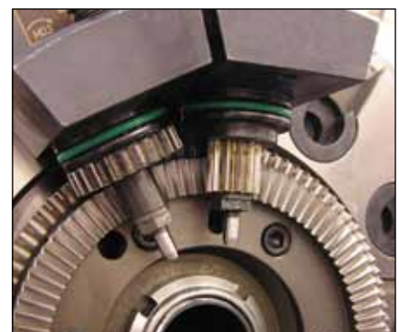
Figure 7—Multimodal Index Traub turning machine with inner and outer face gear rings.
