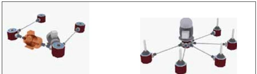
Figure 13—Application examples of Octodrive face gear transmissions: table-adjustment and multiple-lift drive combination.
