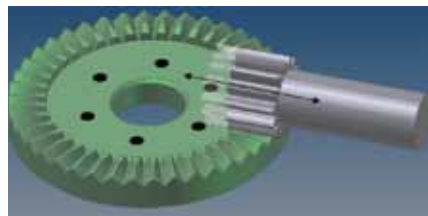
Figure 3—Axial freedom of the pinion in face gear transmissions.
