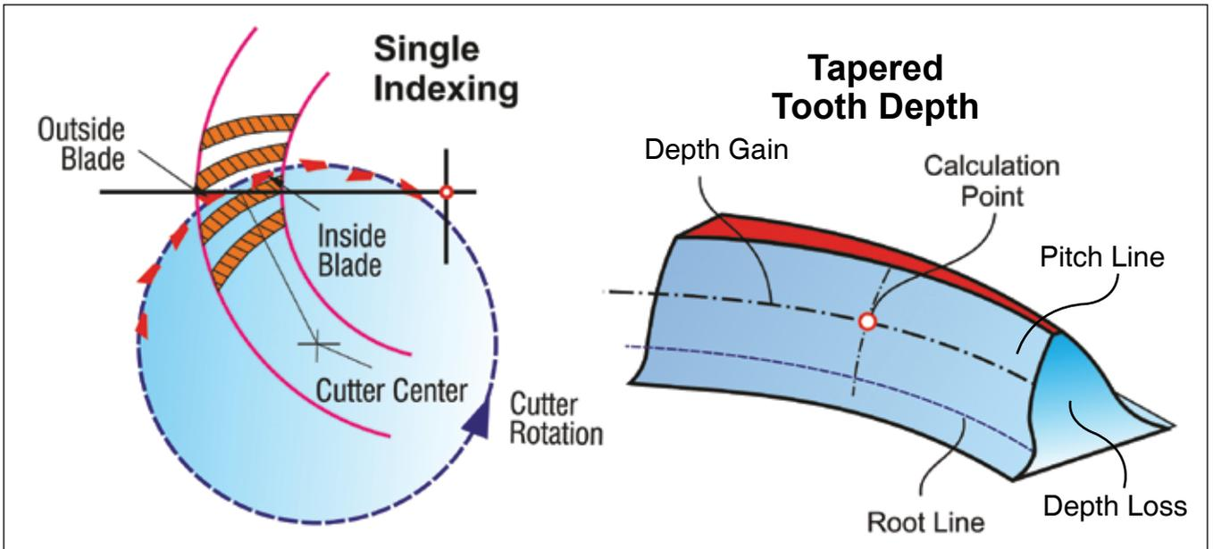
Figure 5—Face milling process and tapered tooth depth.
