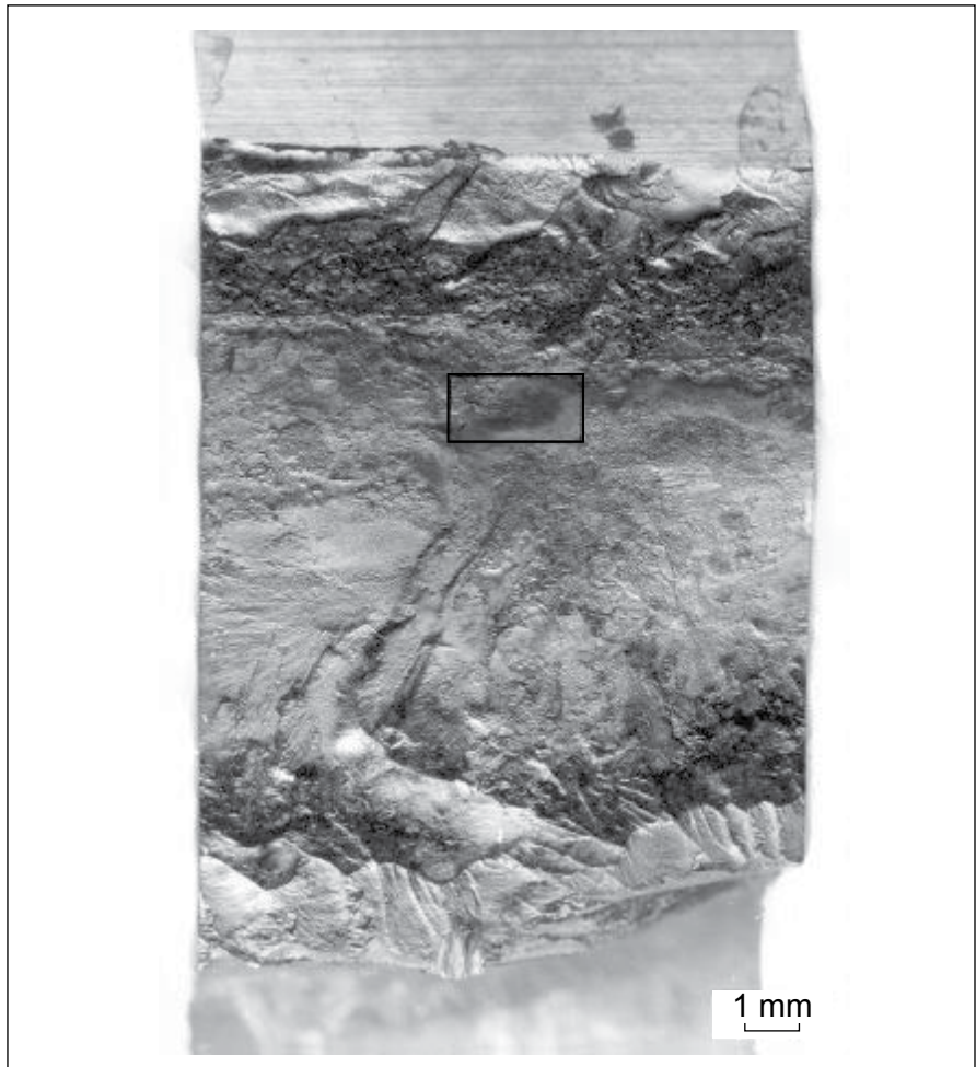
Figure 4—Position of the crack starter PR .
