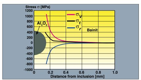
Figure 8—Internal cooling stress at the boundary of a non-metallic inclusion (AI,O<sub> $\alpha$ </sub>).
