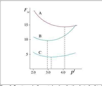
Figure 8—Two-stage epicyclic gear train volume function charts; A = "star" arrangement (Fig. 4); B =planetary (Fig. 5); C =with first differential stage (Fig. 6).
