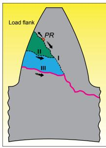
Figure 6—Path of crack.
