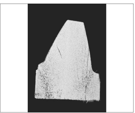
Figure 13—Crack within the volume of the tooth.
