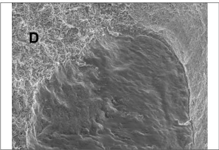
Figure 12—Intense plastic deformation within WEA.
