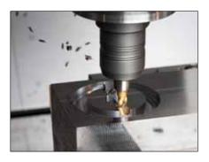
tough milling applications. Twenty-four versions of the shank are available, along with square shoulder and ball nose inserts that have through-tool coolant on all two and three flute designs for excellent cooling and efficient chip removal. Inserts come in two grades for machining all types of materials and E- and M-geometries for a smooth cutting design. Insert diameters range from 0.375" to 0.625" and corner radii are available from 0.0157" to 0.122" to match a variety of design requirements.
