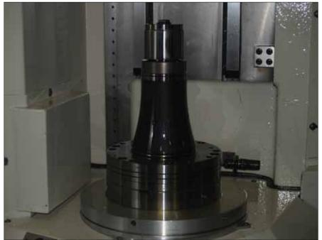
The workholding solution currently in place at United Gear is a series of Hainbuch T213 style mandrels (courtesy of Hainbuch).
