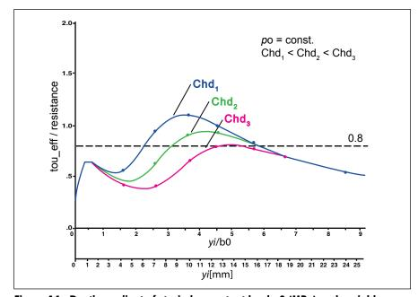
Figure 14—Depth gradient of strain by constant load  $\rho 0$  (MPa) and variable case-hardening depth (mm).
