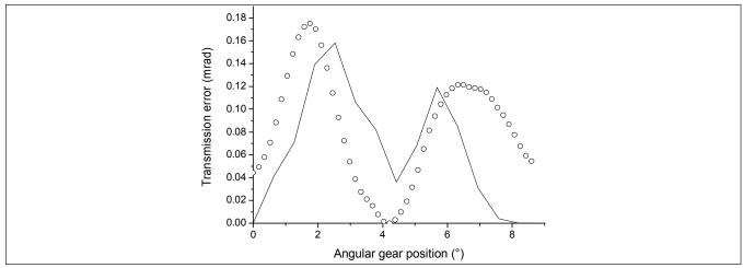
Figure 6—Comparison of measured and simulated transmission error at 25°C, 50% relative humidity, 300 rpm and 10 Nm; (o) = transmission error measured; (-) = simulated transmission error.
