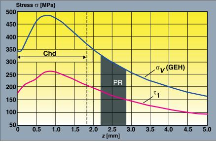
Figure 7—Distribution of equivalent stress and main shear stress over the depth.
