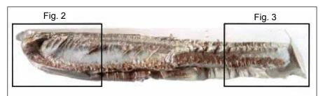
Figure 1—Fragment of a pinion tooth.
