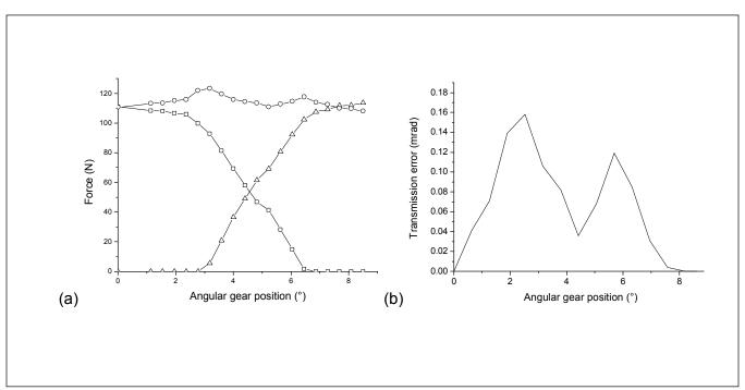
Figure 4—a: Load-sharing model at 25°C, 50% relative humidity, 300 rpm and 10 Nm; (□) Tooth -1; (o) Tooth 0; (Δ) Tooth 1. b: Transmission error at 25°C, 50% relative humidity, 300 rpm and 10 Nm.
