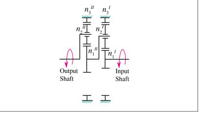
Figure 5—Two-stage epicyclic planetary gear train.
