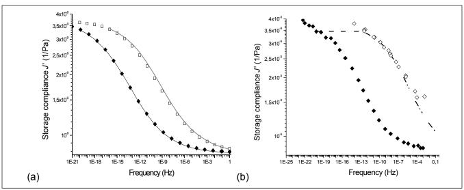
Figure 2—Master curves of storage compliance and fitting with model: a: (\*) dry test at  $T_{ref} = 0^{\circ}\text{C}$ ; ( $\Box$ ) dry test at  $T_{ref} = 30^{\circ}\text{C}$ ; ( $\Box$ ) dry model at  $T_{ref} = 0^{\circ}\text{C}$ ; ( $\Box$ ) humid test (50% RH) at  $T_{ref} = 0^{\circ}\text{C}$ ; ( $\Box$ ) humid model (50% RH) at  $T_{ref} = 0^{\circ}\text{C}$ .
