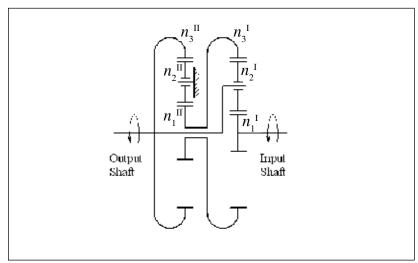
Figure 6—Two-stage epicyclic differential gear train.
