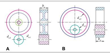
Figure 1—Gear pair volume definition: A = external gearing; B = internal gearing.
