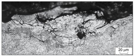
Figure 5—Local separation with radial cracks (Fig. 4).
