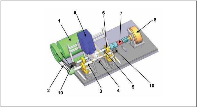
Figure 5—Test bench scheme, showing motor (1), belt (2), rotation axis of pinion (3), gears (4), rotation axis of gear (5), bearings (6), torquemeter (7), break (8), infrared camera (9) and optical encoders (10).
