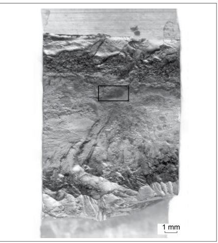
Figure 4—Position of the crack starter PR
