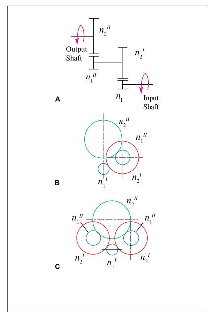
Figure 3—A = two-stage external gear train; B = one-transmission-branch arrangement; C = two-transmission-branch arrangement.
