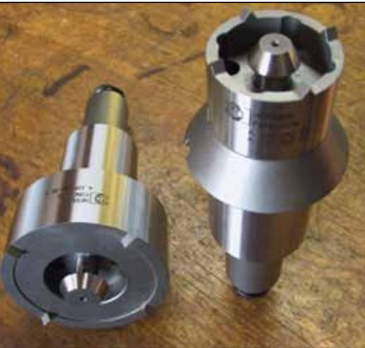
of .00003" to .00007". Also, the center pin and drive disk system can be adjusted to achieve zero runout.
