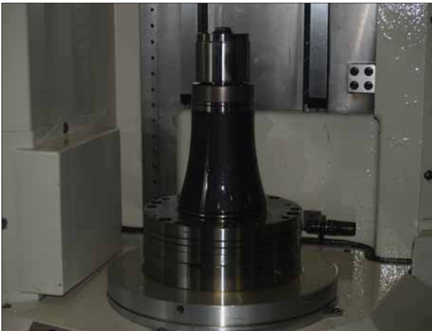
The workholding solution currently in place at United Gear is a series of Hainbuch T213 style mandrels (courtesy of Hainbuch).
