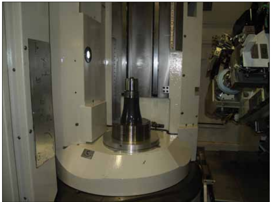
The T213 style was chosen for the ability to have a better cutting profile (tool clearance).
