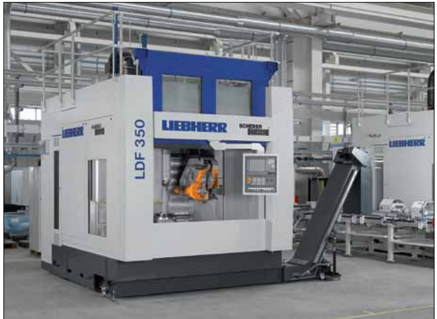
Liebherr's LDF 350 combines turning, drilling and hobbing in a single clamping arrangement.
