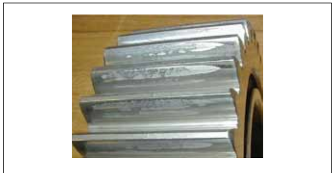
Example of micropitting damage II.
