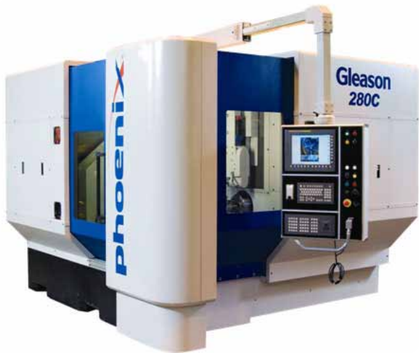
Figure 3 Gleason Phoenix 280C universal bevel gear cutting machine.
