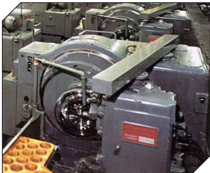
Figure 1 Gleason No. 116 bevel and hypoid gear generator.
