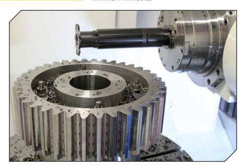
for hard milling heat treated material. "The processing is largely determined by the amount of material removed, how the gear is going to be used, and what AGMA grade is required."
