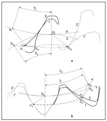
Figure 7 Generating gear shaper cutter profile definition for external (a) and internal (b) gears: 1 and 1′ – gear profile positions; 2 and 2′ – shaper cutter profile positions; 3 – gear pitch circle in mesh with shaper cutter; 4 – shaper cutter pitch circle in mesh with gear.
