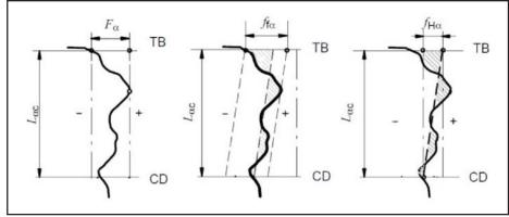
Figure 3 Total, slope, and form errors, AGMA 2015-1-A01.
