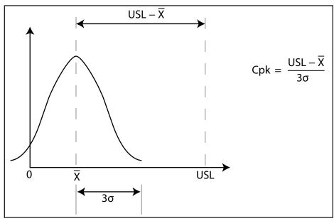
Figure 2 Cpk determination for a unilateral tolerance.
