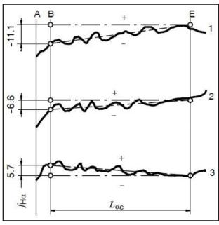
Figure 4 Average and Slope Variation — AGMA 915-1: average = (5.7+ (-6.6) + (-11.1)) / 3 = -4 µm; variation = 5.7- (-11.1) = 16.8 µm.
