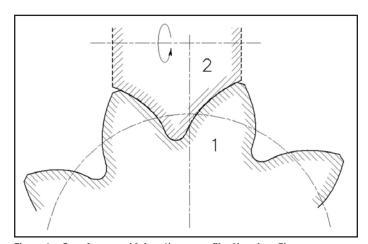
Figure 1 Gear form machining: 1) gear profile; 2) tool profile.
