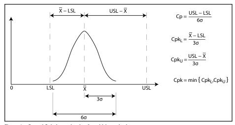
Figure 1 Cp and Cpk determination for a bi-lateral tolerance.
