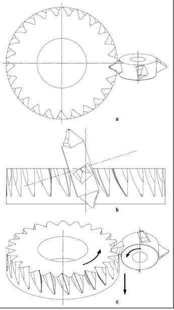
Figure 2 Gear fly cutting schematics: a) top view; b) right view; c) isometric view.
