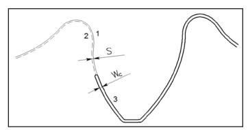
Figure 9 Contour cutting path: 1) nominal (average material condition) gear profile; 2) tool path; machined gear profile;  $W_c$  – cut width; S – tool path off-set.
