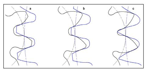
Figure 1 Gear meshes of 10 and 40 tooth gears; a – standard (pressure angle 20°, X-shifts 0 and 0, contact ratio 1.08), b – standard (pressure angle 20°, X-shifts +0.5 and -0.5, contact ratio 1.40), c – nonstandard (pressure angle 22.5°, contact ratio 1.70)
