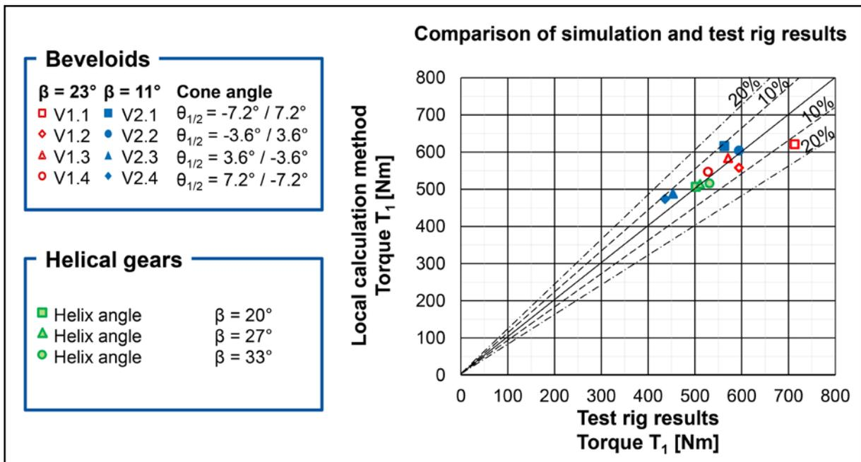
Figure 9 Overall comparison of the simulation and testing results for all tested gears (Ref. 4).
