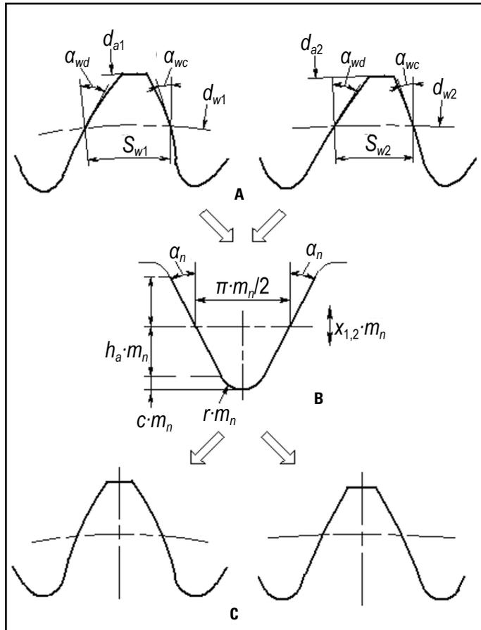
**Figure 3** Definition of symmetric rack for comparable symmetric tooth gears generation based on Direct Gear Design of asymmetric tooth gear pair; A — mating asymmetric tooth pinion and gear profiles; B — symmetric rack; C — comparable symmetric tooth profiles.
