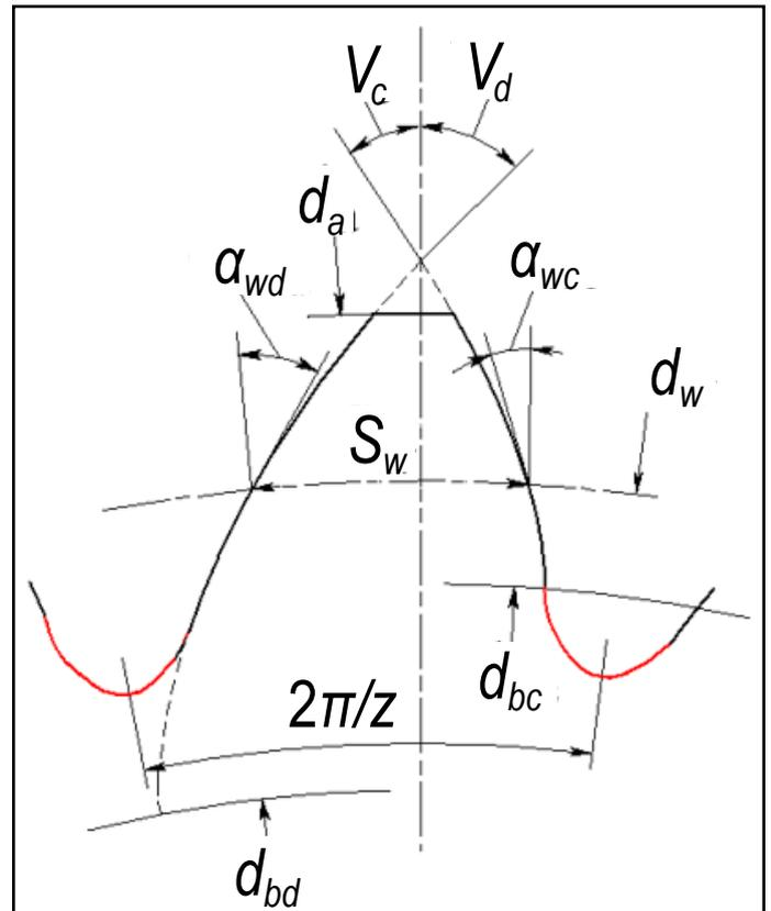
Figure 2 Asymmetric tooth profile (transverse section).  $z$  — number of teeth;  $d_{bd}$ ,  $d_{bc}$  — base diameters;  $V_d$ ,  $V_c$  — involute intersection profile angles;  $d_w$  — operating pitch diameter;  $\alpha_{wd}$ ,  $\alpha_{wc}$  — profile (pressure) angles at diameter  $d_w$ ;  $S_w$  — circular tooth thickness at diameter  $d_w$ ;  $d_a$  — tooth tip circle diameter; symbols “d” and “c” for drive and coast tooth flanks.
