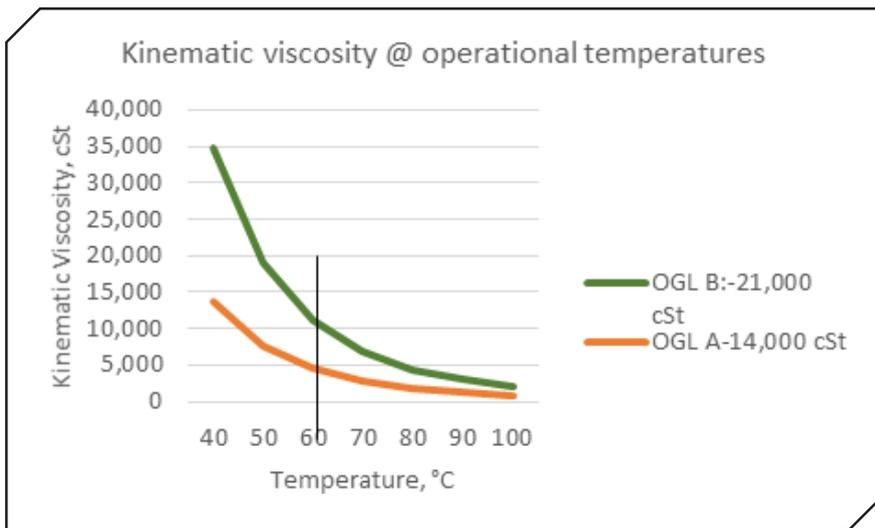
Figure 5 Viscosity of Lubrizol’s OGLs with PP technology at different temperatures.
