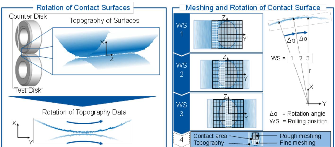
Figure 6 Calculation method of changing pressure distribution within dry rolling contacts.
