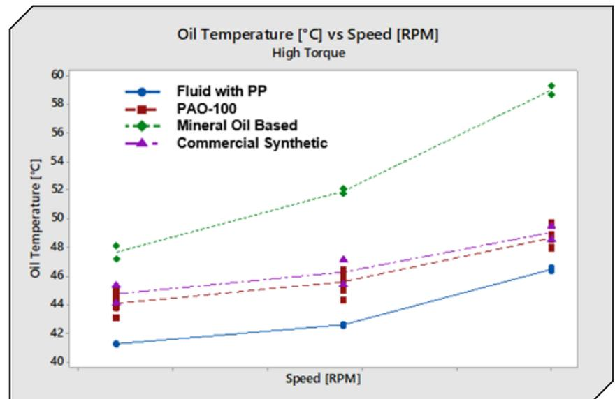
Figure 2 Temperature reduction by worm gear.
