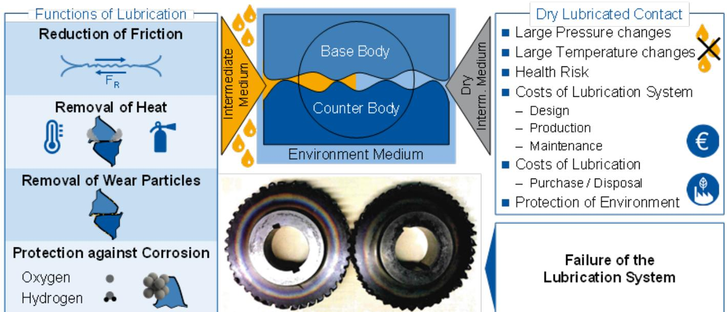
Figure 1 Functions of lubricant in a rolling contact and applications for dry lubrication [Ref 6].
