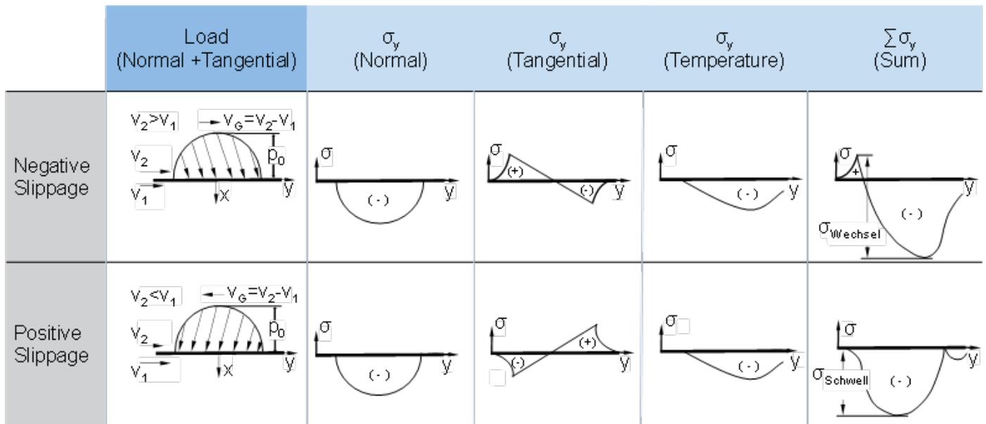
Figure 2 Stresses due to dry lubricated rolling contact [Ref. 1].
