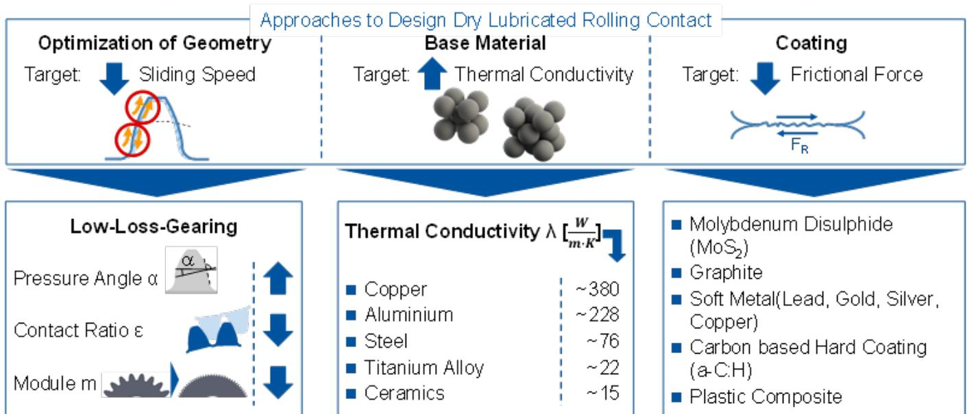
Figure 3 Approaches for dry lubricated rolling-sliding contacts [Refs. 10–11].
