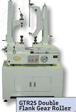
**GTR25 Double Flank Gear Roller**
