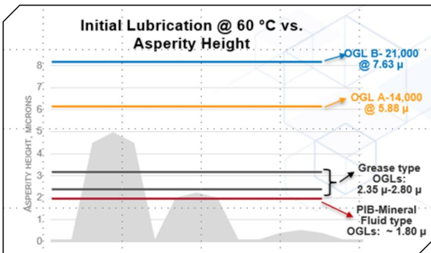
Figure 7 Comparing different OGL tiers film thickness at typical operational temperature.
