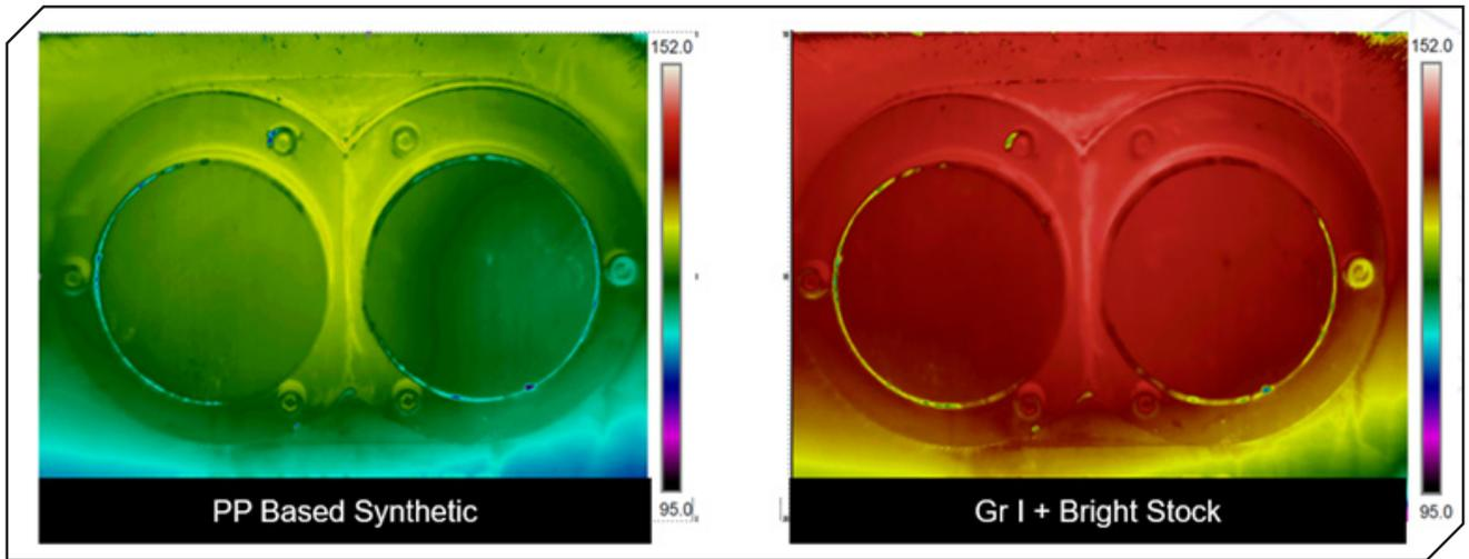
Figure 3 Temperature reduction by FZG rig shows that IGO formulated with PP runs 17 °C cooler compared to conventional mineral oil-based formula.
