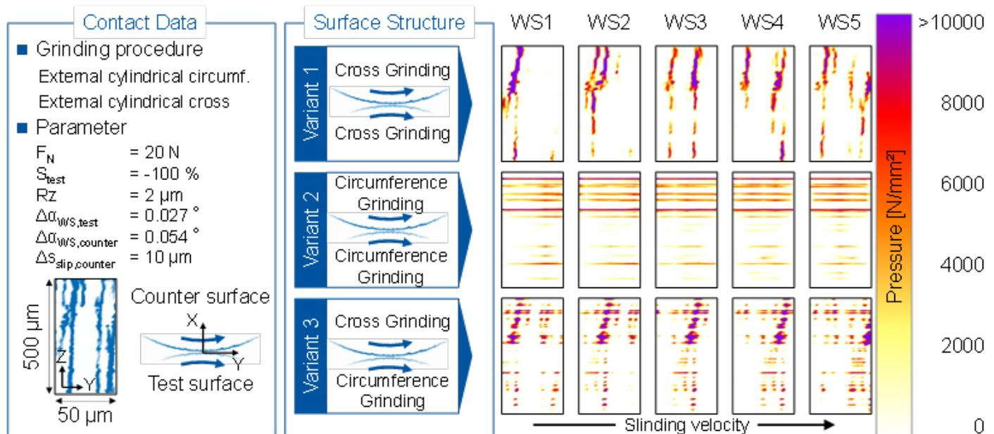
Figure 7 Pressure distribution depending on the contact position and surface structure.
