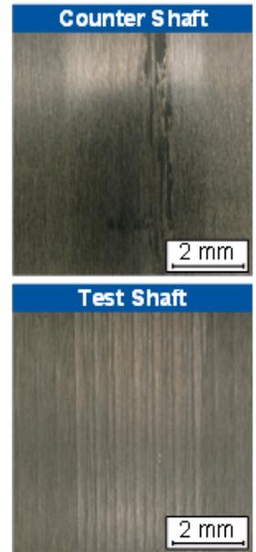
Figure 5 Pre-test pressure ramp-up with dry lubricated rolling-sliding contact.
