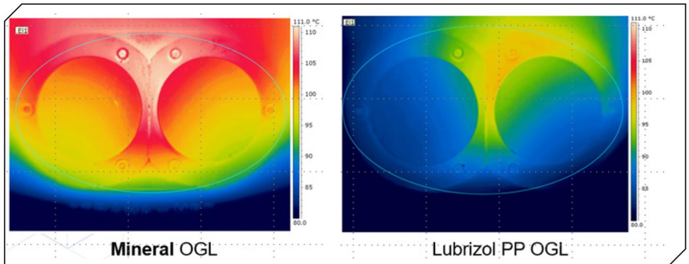
Figure 9 Significant temperature reduction between general market mineral OGL and Lubrizol OGL with PP technology.
