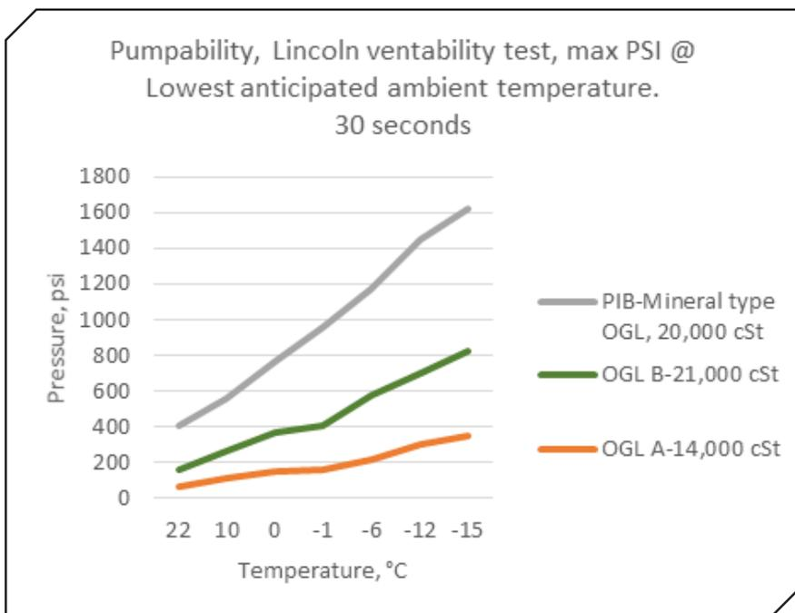
Figure 6 Residual pressure at lowest testing temperature.
