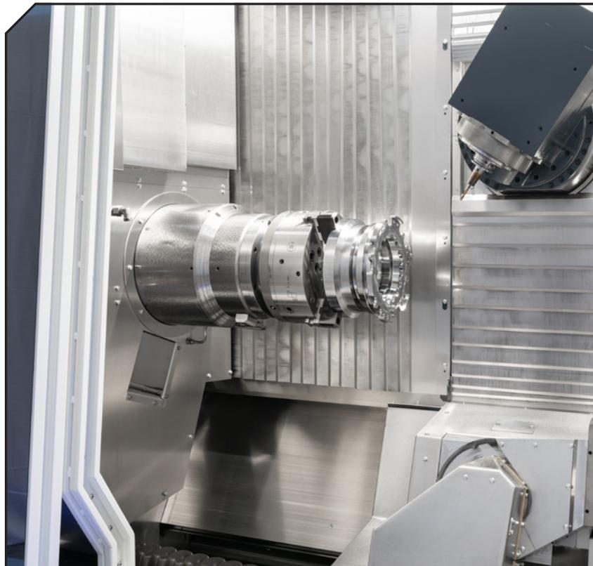
up the tools parallel to machining time and to automatically access the stock in the magazine. Stored tools can therefore be placed in the upper and lower tool holder. With the integrated loading concept, WFL has reduced the space requirement by 50% in comparison to a conventional production cell.
