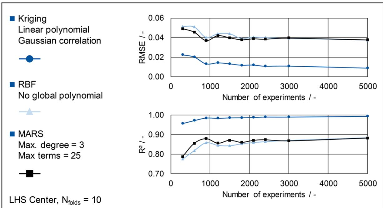
Figure 6 Comparison of different surrogate modeling techniques.
