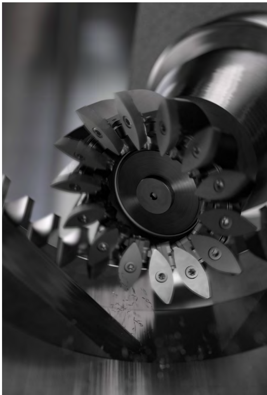
Power skiving is emerging as the fastest-growing method for gear machining for EVs.
