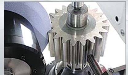
BZ300: A single platform for profile, generating and worm grinding.
