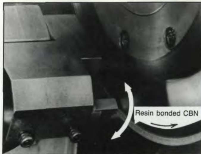
Fig. 4—Attachment for truing of CBN wheel
