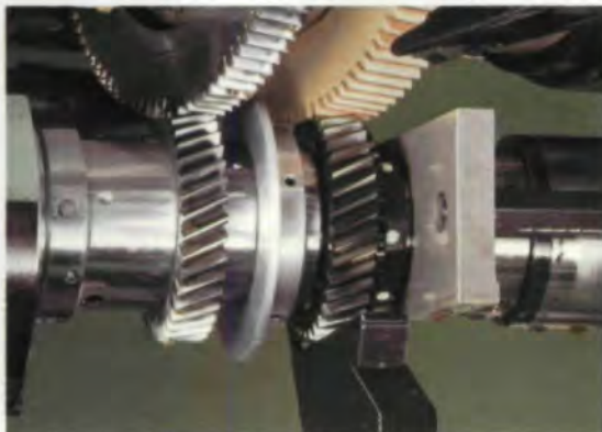
This illustration shows the tool finishing the work-piece gear and the external master gears engaged to control the operation.
